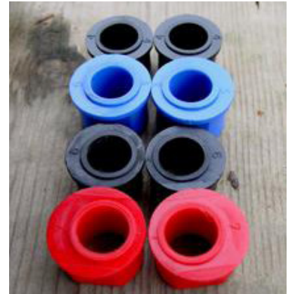
There are different inserts to fit different diameters of rowing and sculling pins. Inserts for different diameter pins are colour coded.
