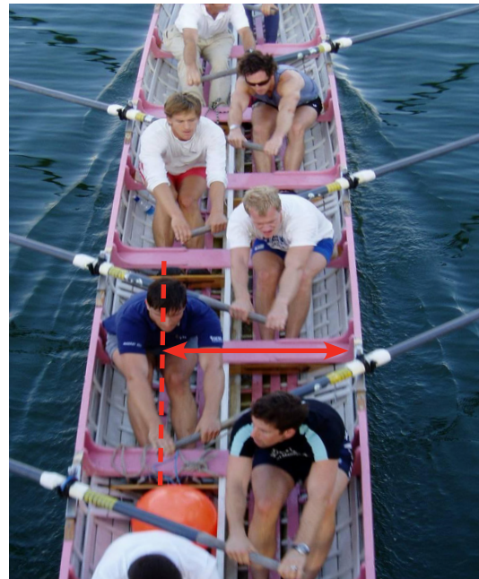
Centre line in a staggered boat
