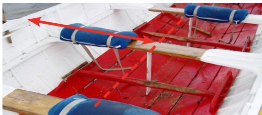
Measuring the distance from pin to the centre line
